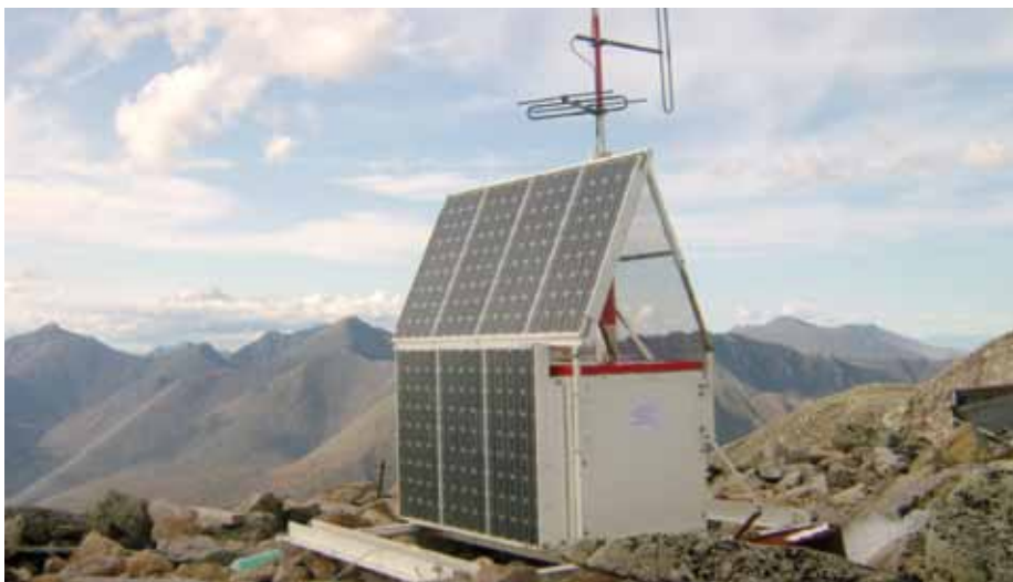
An autonomous VHF radio station in northeastern Siberia.
